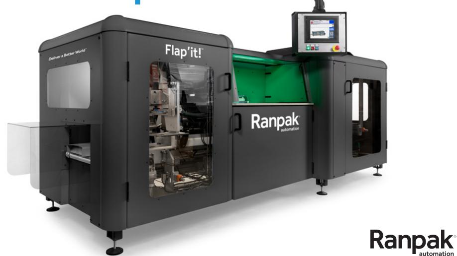
The ergonomic Flap'it!™ system is a highly effective solution that automates the packing of small products.
