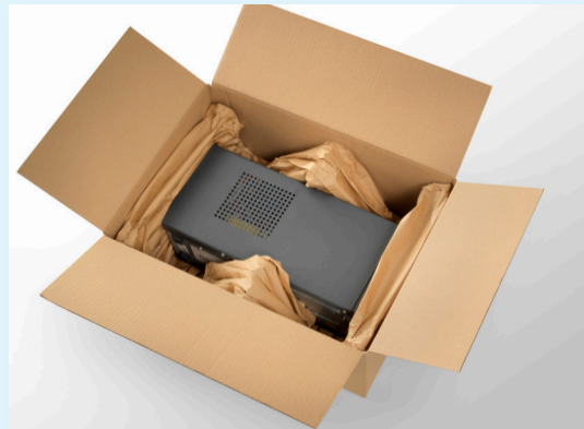
BLOCK AND BRACE
